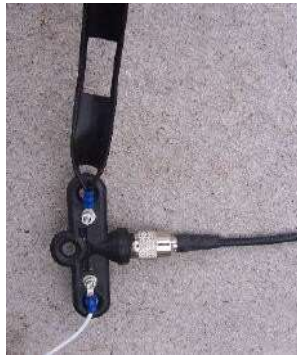
A Typical G7FEK antenna feed point before weatherproofing with self amalgamating tape
