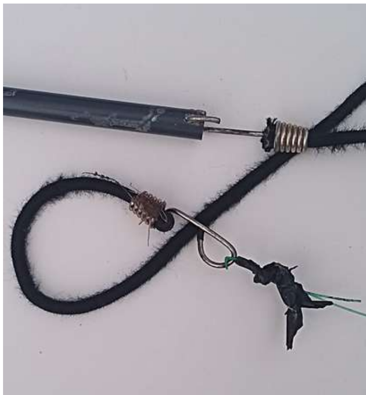
Connected (l-r), the antenna wire, PVC pipe end insulator, “trucker-grade bungee,” and string trimmer support line. After five long years, the wire and the trimmer line didn’t break, nor did the mega-bungee, which got fuzzy but remained sturdy. See text. (NT0Z photo)
