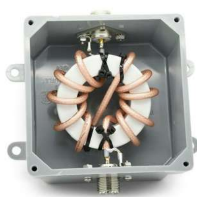
We have found the model 1115U from Balun Designs ($72) to work the best with the Scorpion. It is rated at 3-kW. (Courtesy: Balun Designs)
