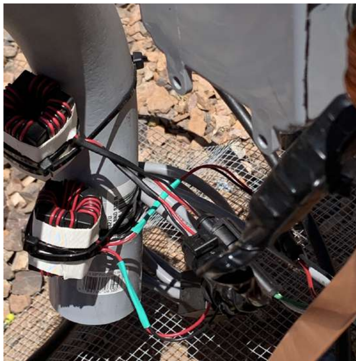
Photo showing the snap-on ferrite cores used on the control cable to prevent RF from going back to the shack via the cable. (KW4H photo)
